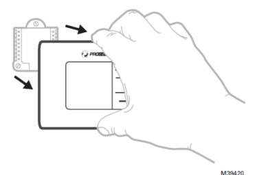
Pull to remove the thermostat from the base plate.
