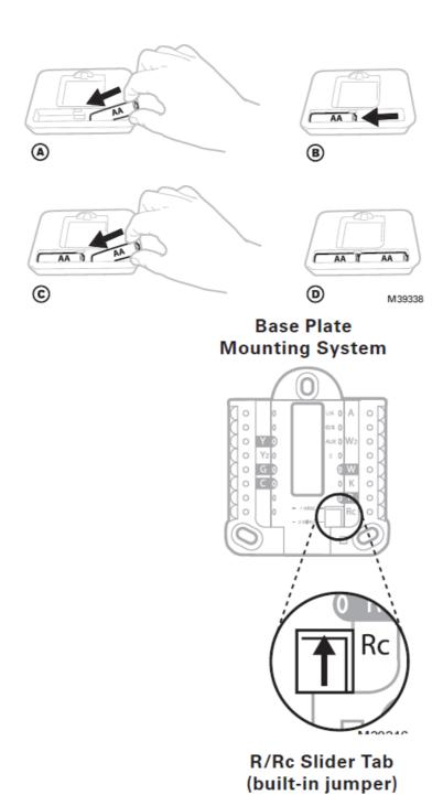
A terminal can be jumped using the Slider Tab. See "Setting Slider Tabs" above.
