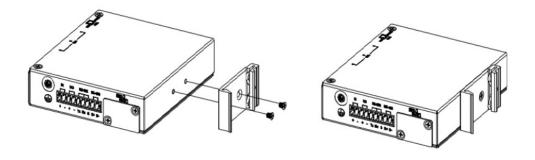
STEP 2: Hook the unit onto the DIN-rail.
