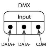
To pass DMX to another device, connect the DMX cable to the DMX Thru port located in the right top corner of the unit. The connector should be wired as depicted in the image below.
