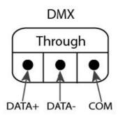
3. Connect the optically isolated DMX signal outputs to DMX links. The connector should be wired as depicted in the image below.
