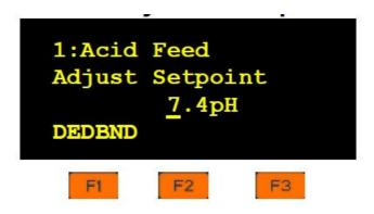
Login with your password if requested, then press .Use the arrow buttons to change the control setpoint, then press to save the new setpoint.
