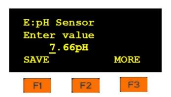
Calibrated. Press NEXT to continue to the next sensor to be calibrated, or press ESC twice to return to the Home screen.
