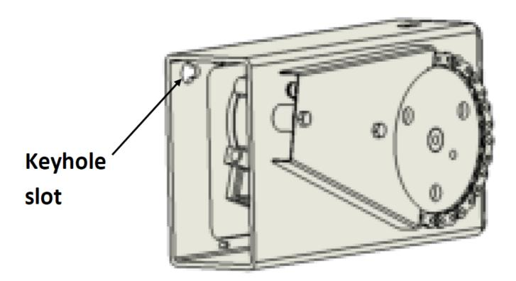
Offer the box into position, fitting the keyhole slot on the rear box surface over the two bolt heads fitted earlier . Next rotate the box upwards into position and locate the front upper keyhole slot onto the casting plate nut loosened earlier. Finally slide the box rearwards to fully locate it.
