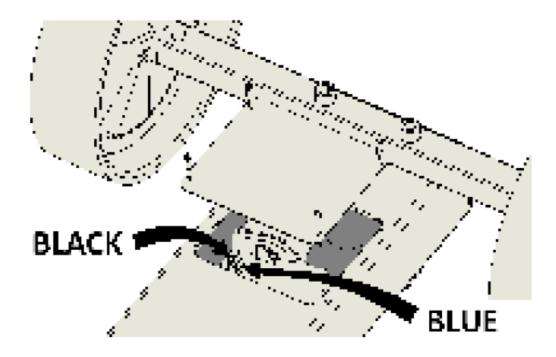
Install the second battery with the terminals facing in towards the handle. For Traps fitted with the large battery tray this step is not necessary as the ring terminals provided on the cable be connected to the appropriate existing battery connector
