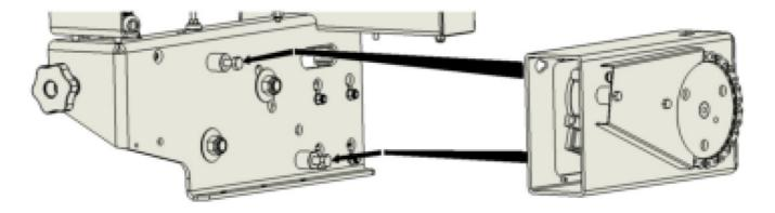
The two main fixing bolts can now be fully tightened, followed by the front casting plate nut. Refit the front and rear plastic caps, taking care not to trap the electrical wiring in the process.
