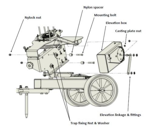
Fit the mounting bolts and spacers to the mainframe mounting holes as shown above, place a NY lock nut on each and hand tighten only, at this stage the bolt heads need to remain protruding.
