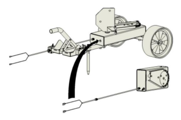
The wiring for the elevation unit is fitted with piggyback type connectors, and should be fitted to the existing motor connectors as shown below.
