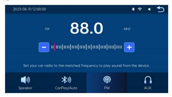
As shown in the picture, click the FM button to enter the FM function: it can send out the sound of the device, receive it withthe original radio, and play it through the original speakers to enjoy the original sound. Matching wires are needed to use it.
