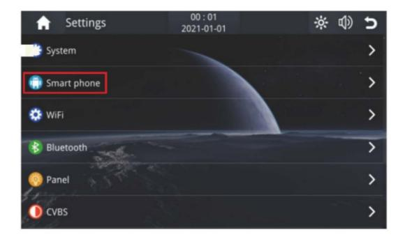
Use your android phone to connect the unit by USB data cable, it will start android phone mirroring.
