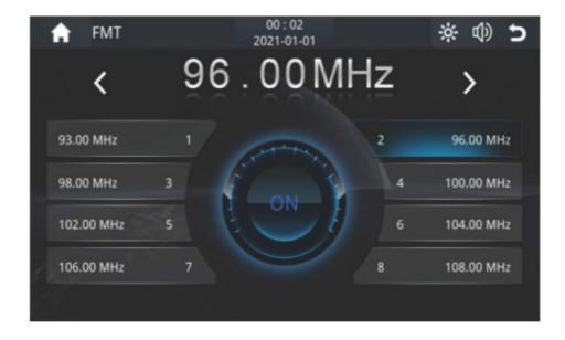
1. By FM radio Recovering- set the same FM radio channel on the unit and your car's radio please avoid using the channel to be (occupied by the FM station)
