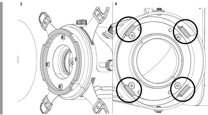
Insert the optic (2-A) and rotate it (2-B) so the marked grooves (3) of the optic coincides with the four marked flaps of the unit (4).
