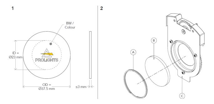
To mount the gobo remove the spring (1) from the gobo holder. Then insert the gobo following the sequence of image 2.
