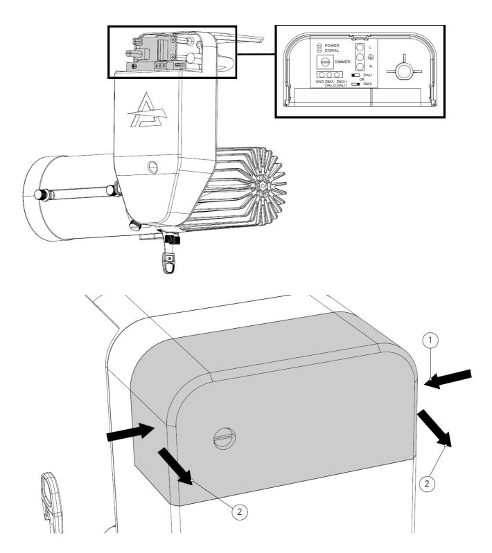
Press down on the sides of the cage (1). Then remove it (2).
