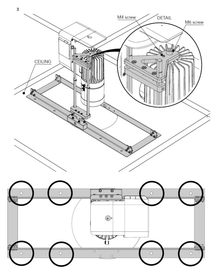
Mount the marked ceiling adapter kit on the ceiling by tightening the screws in the marked points (4). Fit the M6 screw to fix the projector (placed upside down) in the holes provided in the back housing (see detail). Fit the M4 screw to lock rotation.
