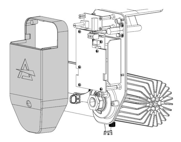
Loosen and remove the marked four screws (2). Then remove the arm housing (3).
