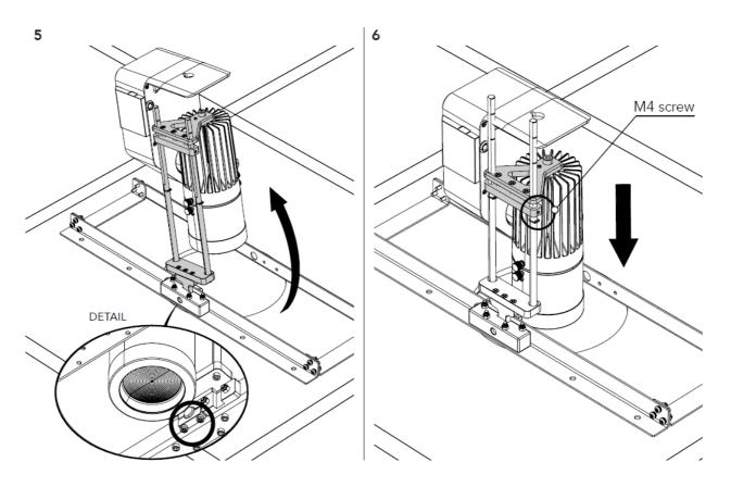
The projector can be tilted with a range of tilt movement of  $-15^{\circ} \div +15^{\circ}$  (5). Tighten the two screws (see "DETAIL") to lock the tilt movement. It is possible to decide the positioning height of the projector by using the marked plate (6). Tighten the M4 screw (6) to lock the vertical movement of the plate.
