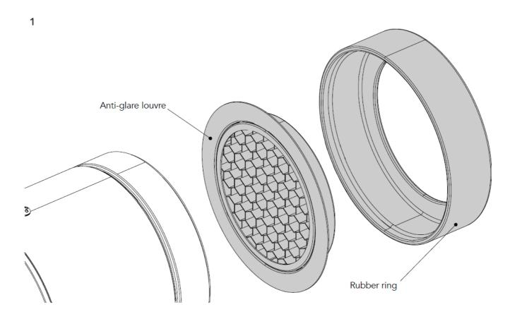
Insert the anti-glare louvre or a filter of maximum size of Ø79 mm into the rubber ring.
