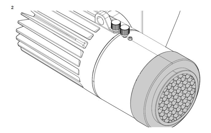
Mount the anti-glare louvre with the rubber ring on the optic.
