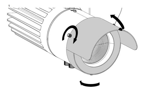
Loosen the three marked knob. Insert the half snoot on the optic and tighten the knobs in the egraved ring.
