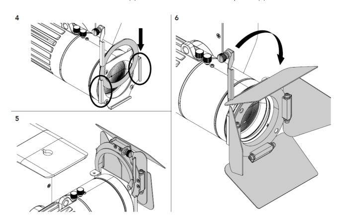
Insert the holder from above throught the track (4). Then insert the barn door (5). Move the marked rod down (6).
