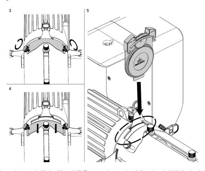
Loosen the two marked knobs of the optic (3). Then move the cover plate (4). Insert the gobo holder into the slot provided on the optic (5).
