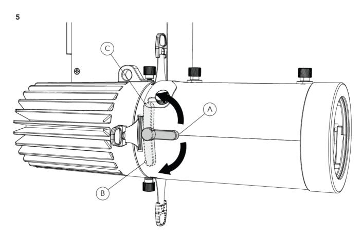
The marked lever in position A allows the locking of the blades. Rotating the lever to position B or C allows the release of the blades. This operation must be repeated for both levers on the frame system.
