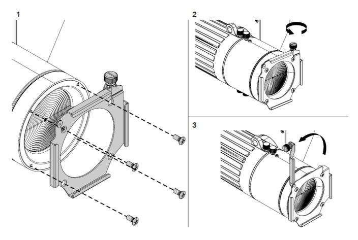
Insert the filter frame mounting the four marked screws into the holes provided on the optic. Rotate the marked knob of the filter frame (2) and and move the marked rod upwards (3).
