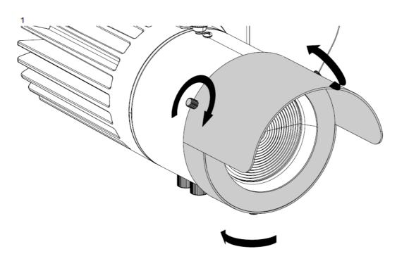
Loosen the three marked knob. Insert the full snoot on the optic and tighten the knobs in the egraved ring.
