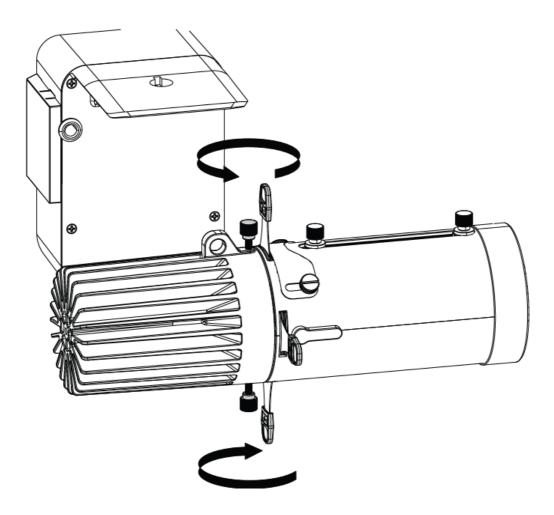
Loosen the two marked knobs on the top and lower of the ECLDISPLAY to rotate the optics.
