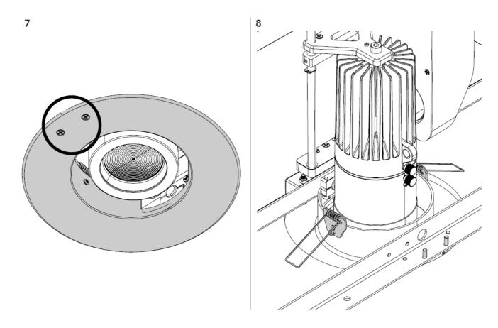
Mount the flange tightening the two marked screws (7) to complete the ceiling adapter kit.
