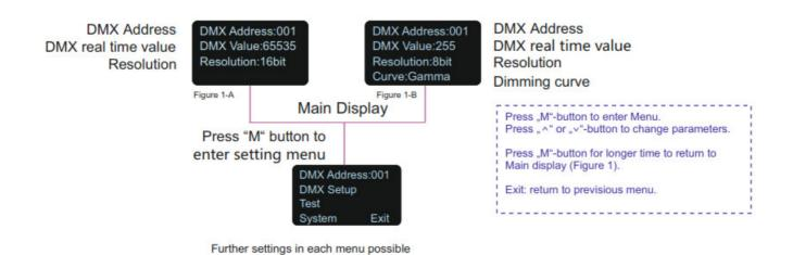
PRO LED DMX PWM DIMMER 1-CHANNEL 2G can start Self-Test-Scenes only when you enter the menu "Self-Test".
