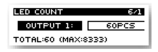
The controller has two digital outputs to control Digital Strips. In this menu you can set the amount of LEDs you have connected or you want to control at each digital output.
