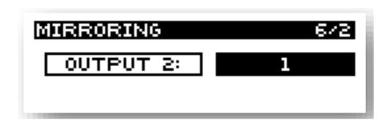
In MIRRORING menu you can set if outputs could be mirrored to other outputs. Here output 2 can only mirror output 1. Output 3 can mirror output 1 and output 2. Output 4 can only mirror output 1, or output 2 or output 3 etc.
