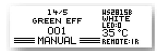
In MANUAL-mode it is possible to use connected Digital Strip without any further controller. All 14 possible settings (look page 22/23) can be changed using UP/DOWN/ESC/ENTER-buttons.
