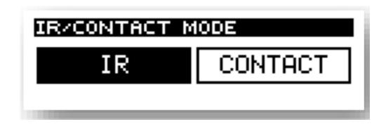
IR input can be used for a IR receiver or as an contact input. When the CONTACT mode is enabled, than in MANUAL mode, if EFF START is signed as ENTER / IR, the effect can be started by a contact.
