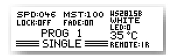
In SINGLE-mode it is possible to use the Pixel Controller PRO as a Stand-Alone-Unit with the connected Digital Strip. You can choose one of the 25 preinstalled programs. Pixel Controller PRO save the last used program and after a power failure starts automatically with this program.
