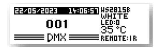
As soon as in main menu DMX has been chosen, the Pixel Controller can be controlled by DMX-signal. As long as no DMX-signal is existing, the start address will blink. The current values for connected LEDs, output order etc. are displayed on right side.
