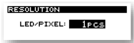
In RESOLUTION-menu you can chose how many LEDs are one pixel. You can enter values between 1 and 100.
