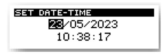
In DATE-TIME-menu you can change the current date and time. This setting is needed for TIMERPRGmode. With the UP/DOWN-buttons you can chose day, month, year, hour, minute or second. The chosen parameter will be displayed inverted. After pressing ENTER-button you can adjust the value With ESC-button you can leave the menu. The current values will be saved.
