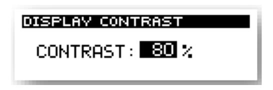
It is possible to adjust the contrast of the display. Higher values means that the display will be darker. Minimum value is 50%.
