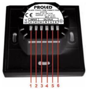
1" and "2": Input Voltage 12 – 24 V DC; "1" is negative pole, "2" is positive pole "3", "4", "5" and "6": Output voltage 12 – 24 V DC, max. 4 A per channel, "3" is positive pole, "4" is connector for red, "5" is connector for green and "6" is connector for blue
