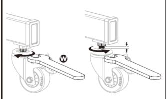
**Note:** If the caster can't touch the ground, loosen the lower nut as shown to adjust the caster to proper position, then tighten the upper nut.
