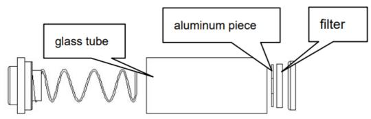
3. Put the spring back into into into the glass tube, then put the glass tube back in position. Press the back holder then the knob will bullet down and become locked automatically.
