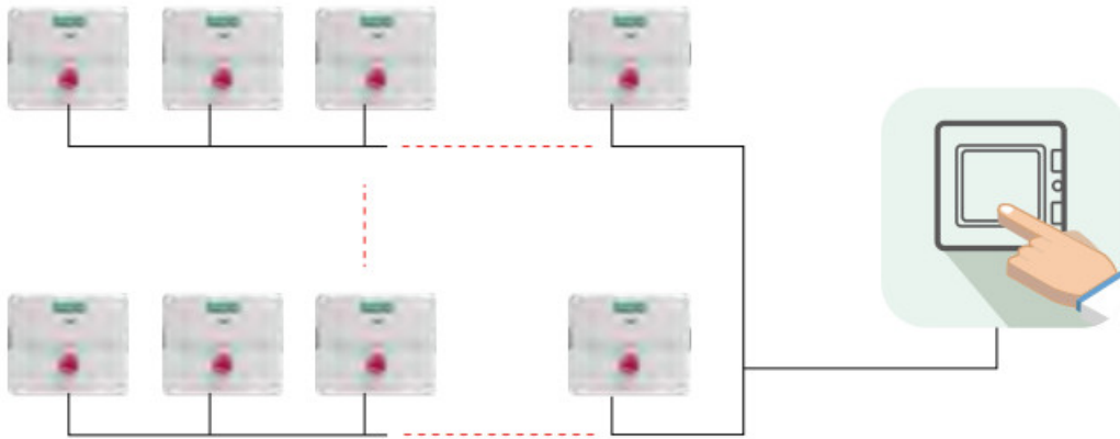
Figure 4.9 Connection diagram of multiple control boxes
