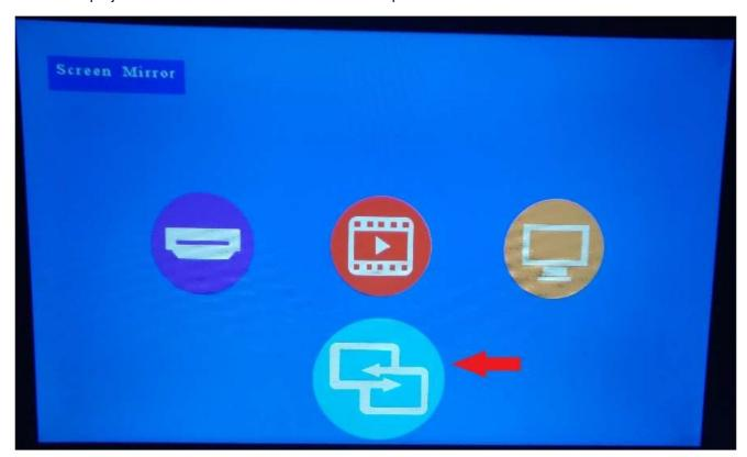
2. Enter the blue interface, and then follow the instructions to connect wirelessly. The IP code in the picture is the network IP address of the projector, and DEVICE is the WIFI of the projector.
