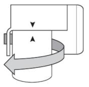
2. Carefully remove the sanitary cap from the top of the new filter.
