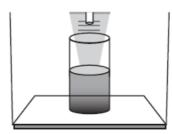
6. Inspect the filter for any noticeable leaks. If leaks are detected, please repeat Steps 3 and 4.
