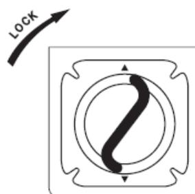
5. Insert the new filter into the refrigerator filter housing and turn clockwise a full 1/4 turn until you feel it stop. The arrows on the filter knob should align with the arrows on the refrigerator.
