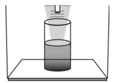
4. Run approximately 2.5 gallons of water from the dispenser periodically to clear the system and to receive a good flow. If the water flow is slower than usual, please repeat Step 3.
