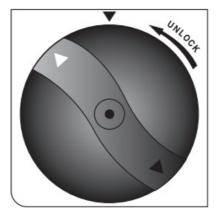
1. Locate your existing filter and remove it by turning the filter counterclockwise. The filter will eject slightly with a clicking sound.
