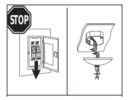
Turn off the power and remove existing fixture
