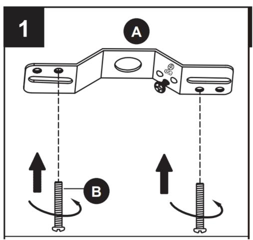
Attach mounting strip(A) to outlet box using two short mounting screws (AA).
