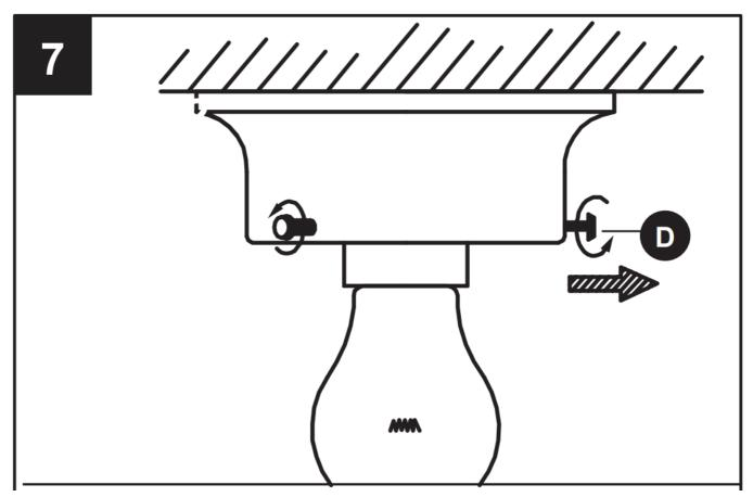
Insert the glass shade (E) into the ceiling plate (C). Tighten three thumb screws (D) to secure glass shade (E).
