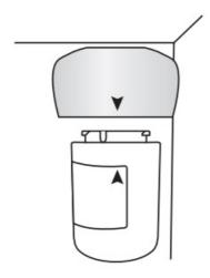
4. Rotate water filter clockwise into refrigerator housing a full 14 turn.
