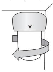
2. Carefully remove the sanitary cap from the top of the new filter
