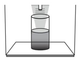
6. Inspect the filter for any noticeable leaks. If leaks are detected, please repeat Steps 3 and 4.
