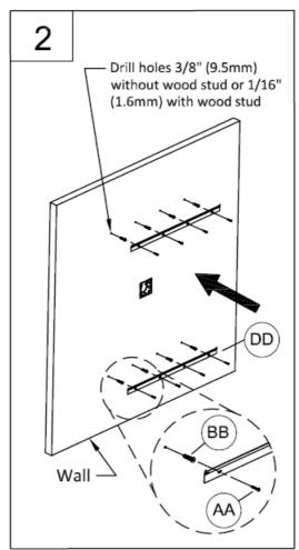
**NOTE:** Wall anchors are required for use in drywall hole locations with no wood stud access. For any pilot holes drilled directly into a wooden stud, the wall anchors are not required.
