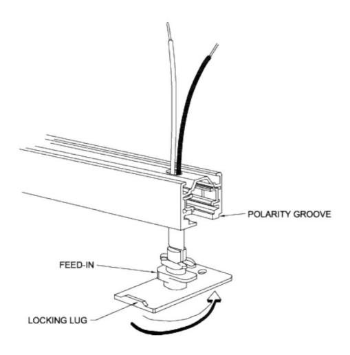
INSERT WIRE AND LIVE FEED-IN THRU HOLE IN TRACK WITH POLARITY GROOVE ON THE OPPOSITE SIDE OF THE LOCKING LUG. TURN LIVE FEED IN A CLOCKWISE DIRECTION FOR  $90^{\circ}$  TO LOCK INTO POSITION. (SUGGEST YOU USE A LARGE PAIR OF PLIERS WITH CAUTION SO THAT YOU DO NOT SCRATCH THE TRACK OR DAMAGE THE EDGE OF LIVE FEED-IN UNIT).
