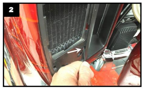
4. Gently pull back on the inside of the rear Lower Fairing cover and pull the Lower Fairing wiring harness through the lower Fairing. Refer to Photos 3 and 4.
