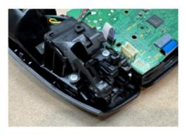
Now you can begin the installation of the smart trigger mod. First, lift and flip over the circuit board from the controller. Be cautious, as there are still wires attached for the rumble motors.
