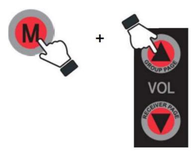
2. STEP 2 Choose between "0" and "8" (The higher number you choose, the higher microphone volume it transmits) "Mic Level" 0 means microphone is mute
