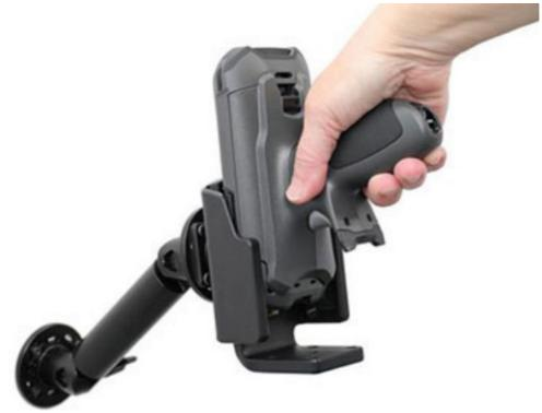
4. **Mounted to the bottom:** Using the included M4 fastener pack, the holder can be attached to any compatible mounting platform. Use the included lock nuts and select the appropriate length fastener to go through the backplate of the holder and the mount then attach using the included lock nuts.
