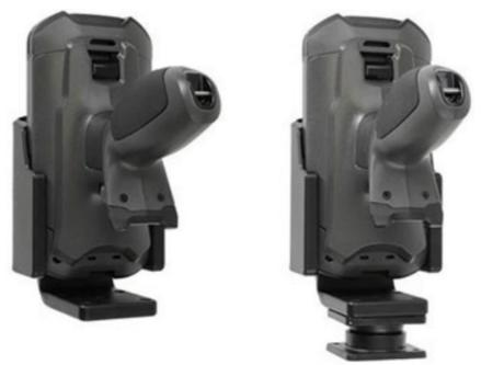
2. **Optional Tilt-Swivel:** The holder and Tilt-Swivel both feature the AMPS hole pattern that is common in a ball, pedestal, pipe, cart, and vehicle mounts. The included self-tapping screws can be used to attach the tilt-swivel to the bottom or the back of the holder to change the docking angle up to 15 degrees in any direction.
