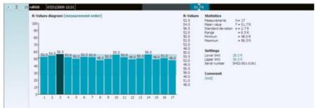
In this example, the third reading can be clearly seen to be outside the limits.
