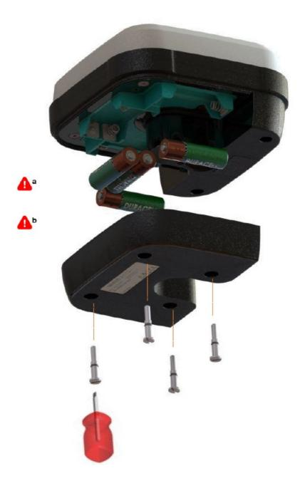
Ensure correct polarity when inserting the rechargeable AA batteries. Alternatively, you can use non-rechargeable AA batteries. Warning: do not charge non-rechargeable AA batteries!
