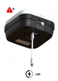
Green: charging; off: finished charging; orange: almost fully charged, temperature limit exceeded (wait or disconnect); red: AA cells incorrectly inserted or temperature limit exceeded (wait or disconnect). Do not let the battery pack discharge for longer than one month.
