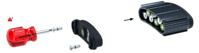
**a** c. During storage for longer than 3 months, do not leave the batteries in the battery pack. Remove by following the reverse procedure.
