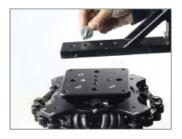
• Loosen the side lock lever & insert your gimbal then again lock the lever to secure it. If ronin plate look loose then tighten the side allen
