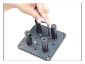
• Now attach this Middle Base Plate with Isolator Plate and tighten the bolts accurately with allen key, as shown
