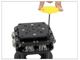
• Then remove bolts and one wire set from Vibration Isolator plate.
