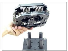
• Now loosen 4 corner bolts of Middle Base Plate and remove Rods as shown in image.
