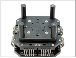
• Turn Isolator upside-down & loosen the bolts to remove Isolator with Base Plate.
