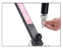
• Detach Locking clamp from the central fork, mount central fork to tripod bowl, again attach Locking clamp for a secure connection.
