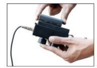
• Attach head cable to cable connected to gold pan-tilt head as shown below.
