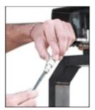
• Loosen the knob on the rear section, remove closers from the weight bar and insert it into the slot on the rear section. Retighten the knob to ensure a slip-free connection.
