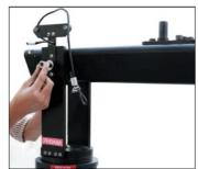
• Slide in (8th) section to the rear to join the 7th section. Install the Allen screws to the joining holes of both sections and tighten them.
