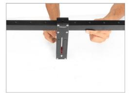
• Adjust the cross bar height by sliding it along the side bar.
