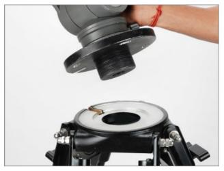
• After mounting the fluid head (Not Included) on the Mitchell Tripod Stand, tighten the Castle ring from the bottom as shown in the image.
