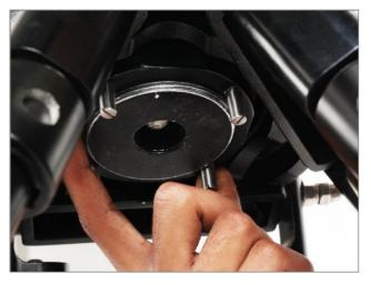
• Remove the Fluid head top plate (Not Included), by pushing the Push pin of the fluid head then attach the plate to the bottom, matching the camera's threads.
