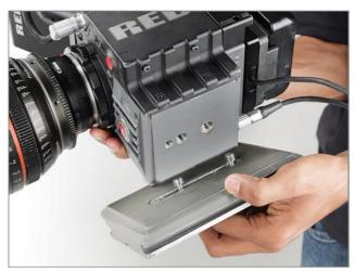
• After attaching the Fluid head plate (Not Included), tighten it properly using a screwdriver. Then mount the camera (Not Included) onto the fluid head by sliding.
