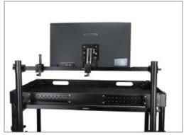
• After mounting the monitor system, properly tighten the knob.
