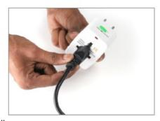
• Attach the 4-pin Power Cable with the Joystick Controller.
