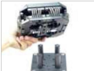
• Now loosen 4 corner bolts of Middle Base Plate and remove Rods as shown in image.
