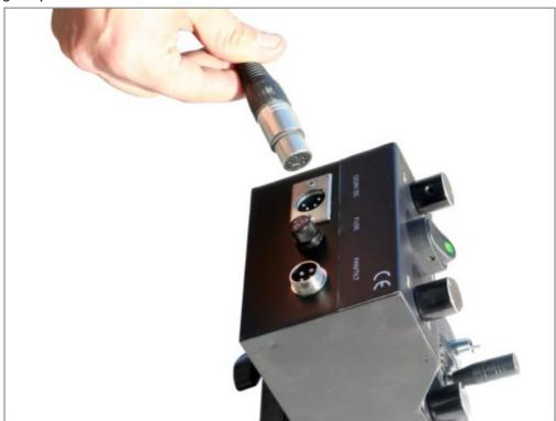
• Install 12 volt AC adapter (4 pin XLR) in the socket of Joystick Box.
