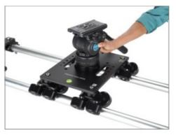
• After mounting the fluid head (Not Included) on the bowl, secure it by inserting the Conversion ring & locking knob from the bottom side of the Dolly.
