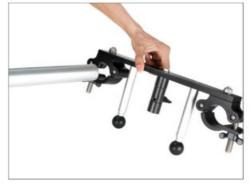
• After properly inserting the track rail into the clamp, secure it by tightening the knob.
