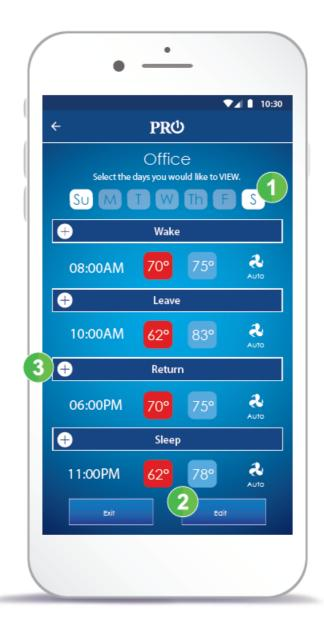
**Note:** The T701i is shipped as a non-programmable thermostat. If you would like to use this feature, you must first turn scheduling on through the thermostat menu located in the top right corner of the thermostat home screen.
