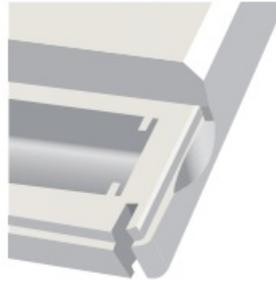
Replace with 2 AA Alkaline batteries.
