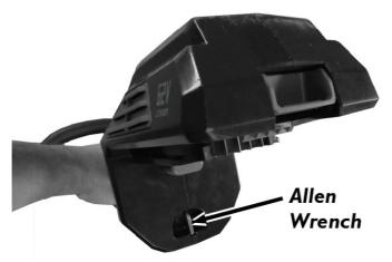
8. Turn the Trimmer around. Set the Protective Cover onto the Mounting Post and secure with 4 Screws using a 5mm Allen Wrench (Figure 4).
