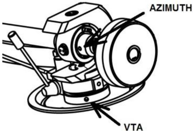
With the aid of a good magnifying glass adjust the needle until it is vertical in the groove (i.e. perpendicular to the record's surface). Ideally, this should correspond to the top surface of the cartridge body is parallel to the record surface, but in practice, this is often not the case. When you are satisfied that the needle is vertical, retighten the screw carefully.
