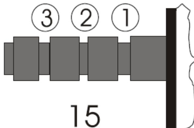
Hang the loop of the thread of the anti-skating weight in the groove of the anti-skating stub (15) corresponding to the downforce applied to your cartridge and hang the thread in the groove of the wire support (17).
