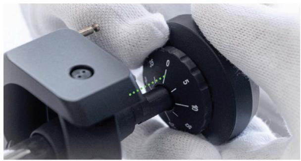
• Turn the counterweight counterclockwise 16 until the scale reads roughly 18.
