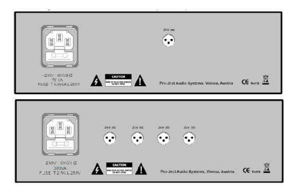
Connect the power cable to the unit and to the mains. Then use a special supplied cable to connect the Power Box RS Uni with the suitable Pro-Ject product. The original power supply is then no longer required.
