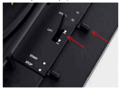
10. elect the playback speed and move the tonearm lift to the upper position.
