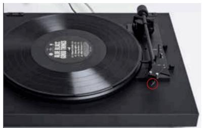
9. Put a record on the turntable & carefully remove the stylus protection cover.
