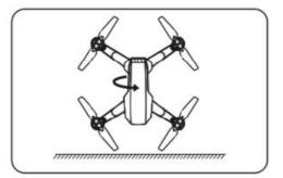
Press and hold the geomagnetic correction button until you hear a bleep and the front and rear lights of the drone flash. Pick up the drone with the base facing the ground and rotate until you hear a bleep. The front lights will flash and the rear light will stay solid. Face the drone's camera to the ground and rotate until a bleep is heard, when the rear light flashes compass correction is successful.
