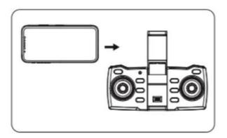
Open the phone holder and place the phone securely onto the controller.
