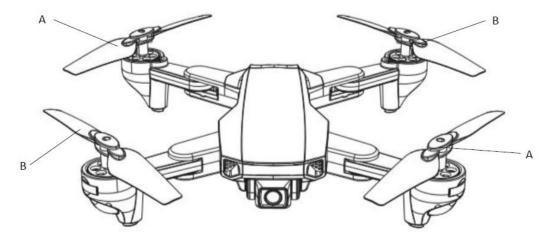
Should one of the fitted propellers become damaged, it can be replaced, by removing the screw from the top of the propeller before sliding the propeller off the motor shaft. Refitting is the reversal of removal. It is important for the correct blade to be placed on the correct motor or the aircraft will not fly correctly. Each blade is marked with an A or B on the top to indicate which motor it corresponds to.
