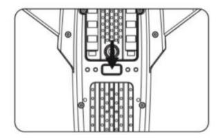
Power on the drone by pressing the power button on the underside of the aircraft. Then press and hold the power button for 3 seconds, the light will flash for around 3 seconds.
