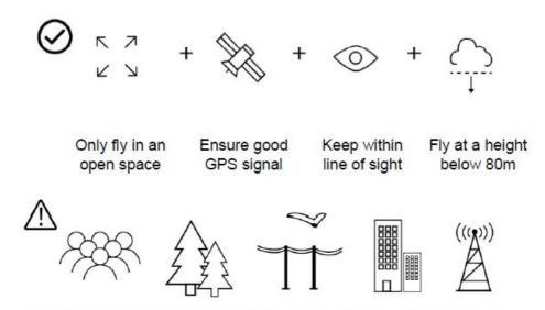
When flying ensure that the drone is kept away from other people, trees, electric wires, buildings, airports or signal transmitting tower etc.
