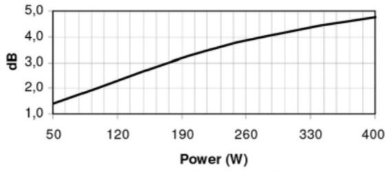
Note: These losses are calculated from a five minutes AES power test applying band limited pink noise (25 - 1200 Hz). The loudspeaker is free-air standing.
