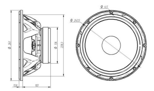
Nominal diameter 250 mm (10 in) Rated Impedance 16  $\Omega$  Minimum impedance 4  $\Omega$  Power capacity 400 W (RMS) Program power 800 W Sensitivity 96 dB 1W / 1m @ ZN
