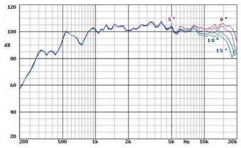
**Notes:** dispersion measured with two waveguides coupled to a  $90^{\circ}$  x  $5^{\circ}$  horn in anechoic chamber, 1w @ 2m. All angle measurements are from the axis  $(45^{\circ}$  means  $+45^{\circ}$ ).
