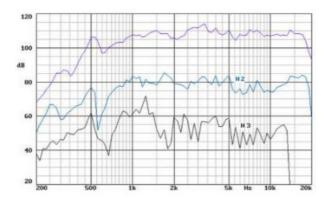
Note: on axis frequency response measured with 2 waveguides coupled to a  $90^{\circ}$  X  $5^{\circ}$  horn in an anechoic chamber, 1 w@ 1 m.
