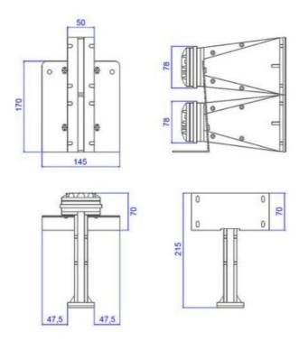
GTA 2X8 L.A. is also composed by two (2) Beyma compression drivers of 50 W RMS, coupled to a waveguide. Specially designed under our own parameters for the best performance of the system.
