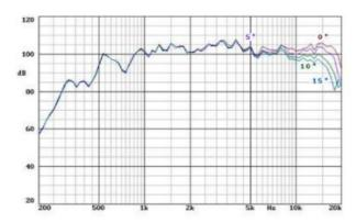
Notes: dispersion measured with two waveguides coupled to a goo x 5° horn in anechoic chamber, 1w@ 2m. All angle measurements are from the axis ( 45° means + 45° ).
