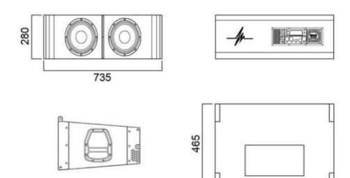
Inside the GTA 2X8 L.A. is composed by two (2) Beyma speakers of 8", 300 W RMS. Specially designed under our own parameters for the best performance of the system.
