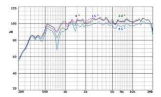
Notes: dispersion measured with two waveguides coupled to a goo x  $5^{\circ}$  horn in anechoic chamber, 1 w@ 2m. All angle measurements are from the axis ( $45^{\circ}$  means +  $45^{\circ}$ ).
